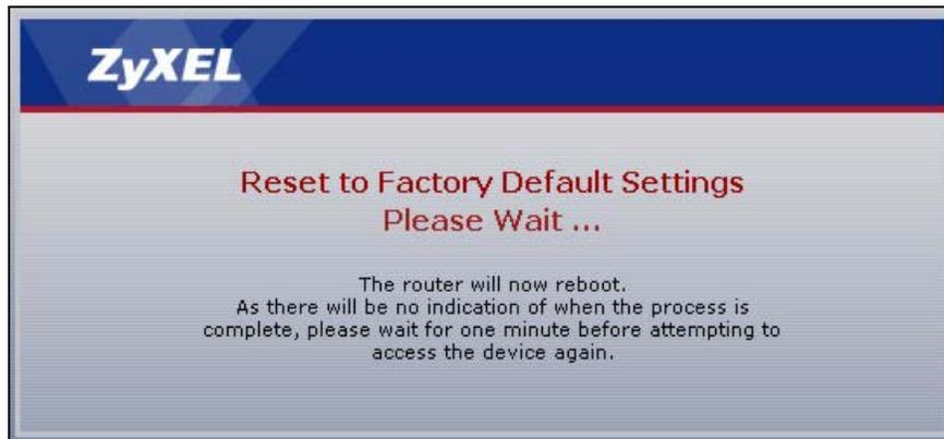
You can also press the **RESET** button on the rear panel to reset the factory defaults of your ZyXEL Device. Refer to [Section 2.1.2 on page 51](#) for more information on the **RESET** button.
